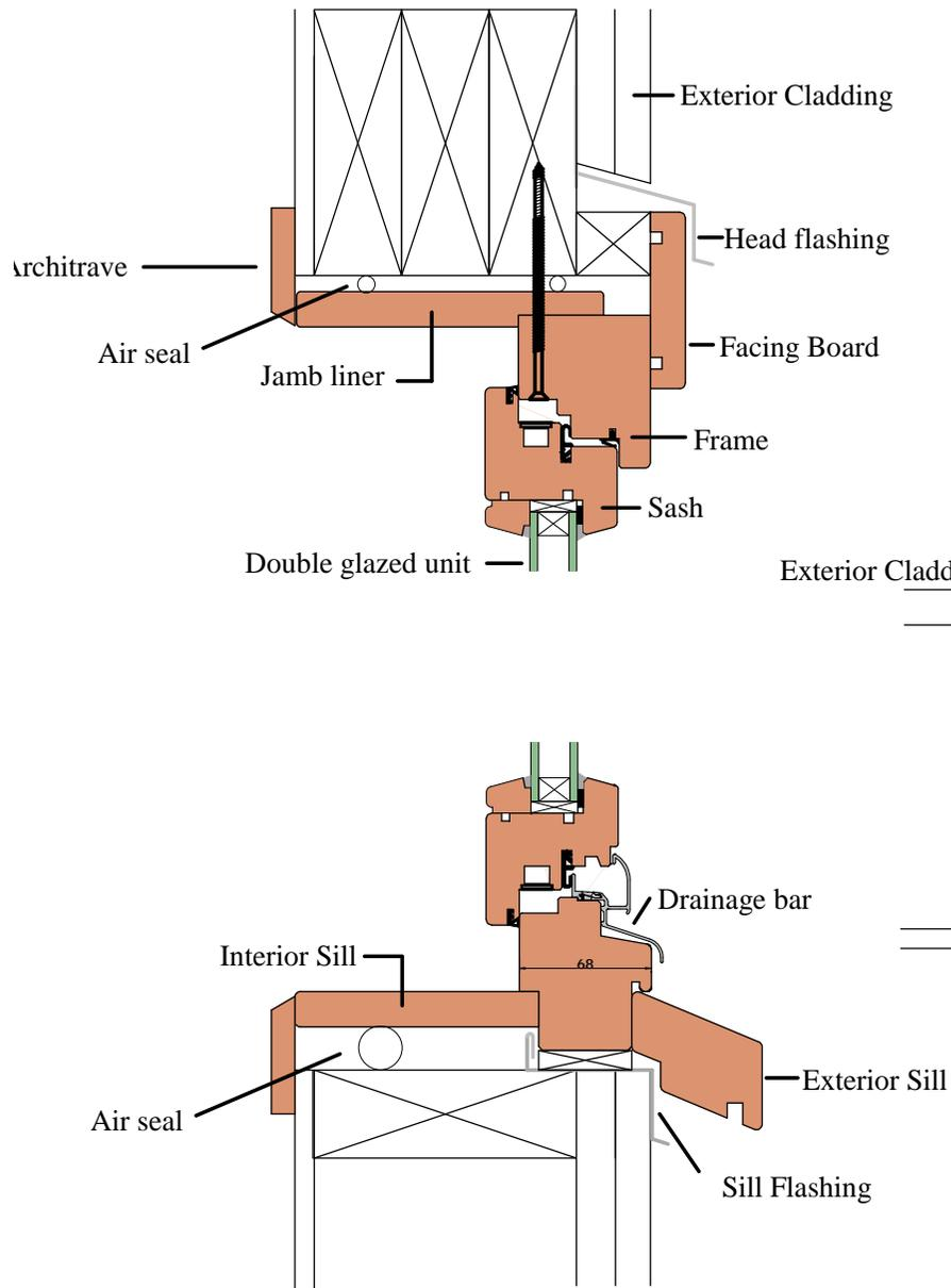
Basic installation with exterior of frame flush with exterior of cladding. Timber jamb liner/reveal.
